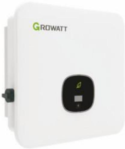
The Growatt MOD 5000TL3-XH Three Phase Hybrid Inverter is a small size three phase grid connected inverter with a power up to 5000W and has 2 MPPT charge controllers. It is capable of working connected to the grid while also being connected to batteries to store excess energy. It is important to note that with this product, it is not necessary to purchase batteries at the beginning of the purchase, which considerably reduces both the cost of the installation and the amortization time.
